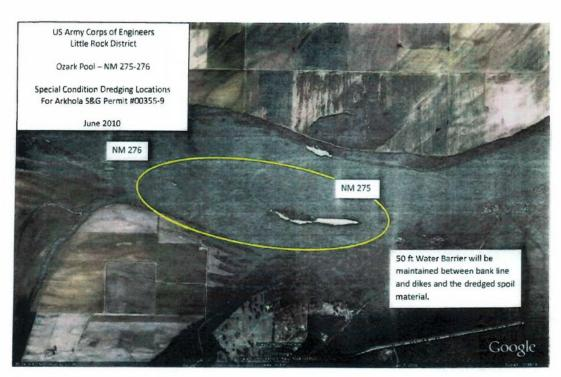
Figure 2. NM 275-276 Right Bank: Dredging will be allowed in this vicinity to remove excess material to establish a minimum water barrier of 50 feet.
